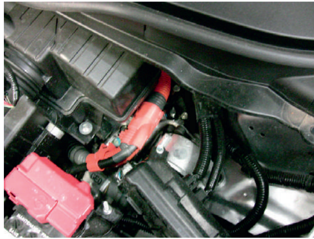
Figure 2.345 High-voltage cables are always orange
